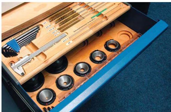
Design Cart型工具车抽屉的插件/ Insert for drawer for Design Cart Power Clamp 和 Power Clamp Preset 型热缩机用/For Power Clamp and Power Clamp Preset
