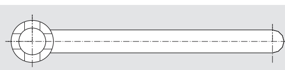
用于 Ø 16–60 面铣刀端面锁紧螺钉或组合壳铣刀用扳手/Wrench for tightening bolts for face mill arbors and combination shell end mill adapters Ø 16–60
